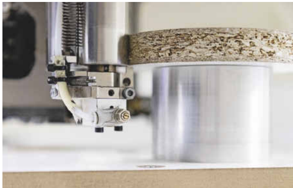
Gut in Form: das Kantenanleimaggregat PowerEdge Pro Duo
